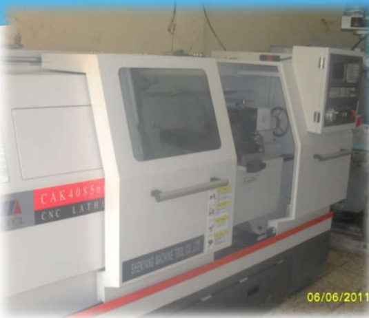
CNC Lathe Machine SENYANG , 10 Inchx800mm 3500 rpm
