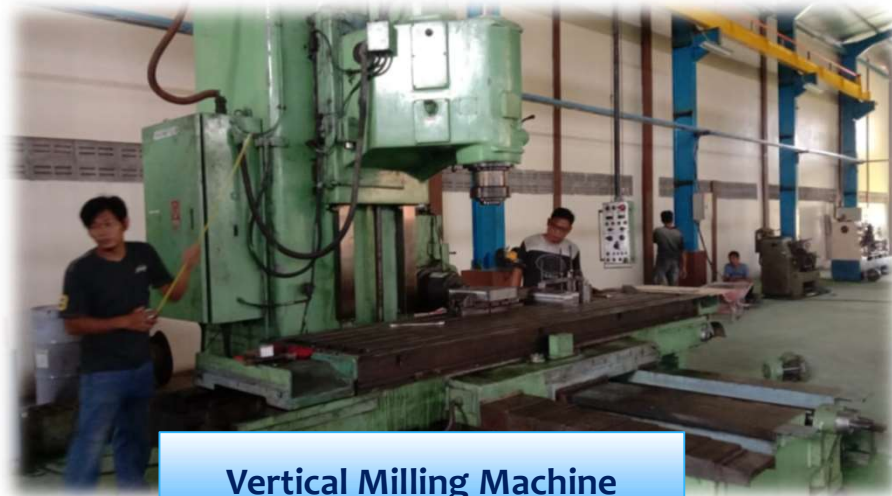
Milling Machine Cap 1000 x 4000 mm
