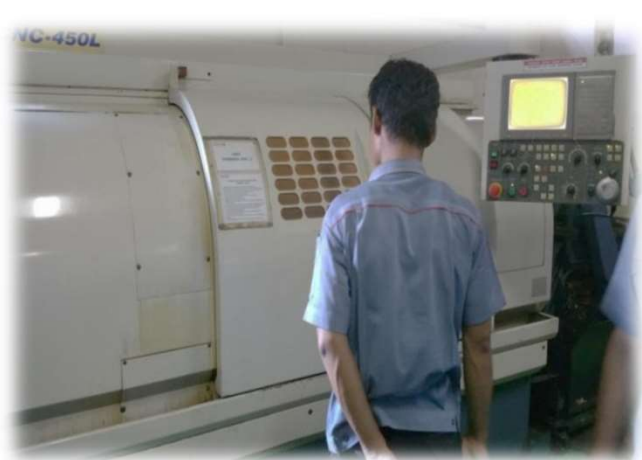
CNC Lathe Machine LIOUYHSING , Taiwan 2005 10 Inchx800mm 3500 rpm
