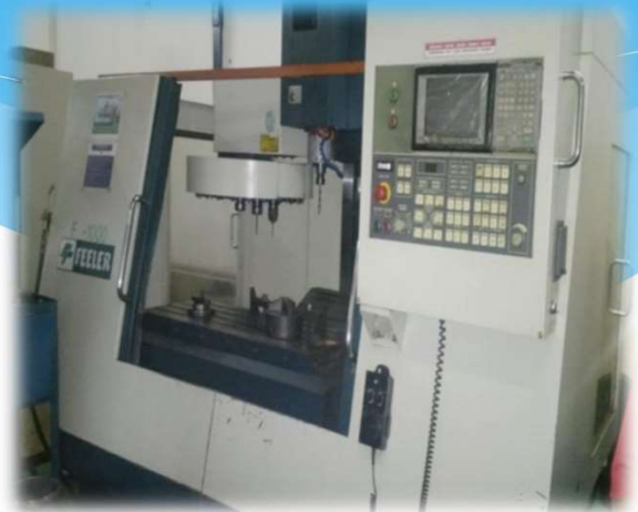
Machining Center Feeler F-1000 , Taiwan 2005 Travel 600x1000mm , 3 Axis 10.000 rpm
