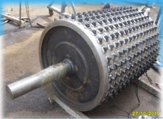
Coal Crusher 200 ton/hour
