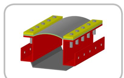
Fabric expansion joints mounted on parallel flanges with insulation bolster, typically used in plants with:
