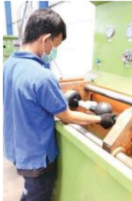
Hydro Test (High Presure)
