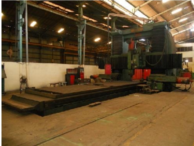
MULTI FACE MILLING MACHINE L 8000 mm x W 2500mm ..
