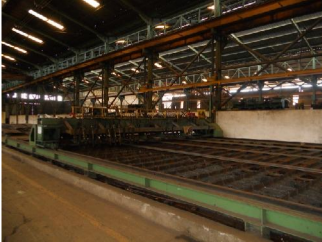
MULTI TORCH FLAME PLANNER 6 mtr x 20 mtr, cutting.
