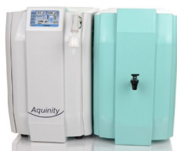
Acquinity 2 - Ultra Pure Water Purifications with Storage Tanks (10/35/70 L) for Analytical & Life Sciences. Requires Tap Water
