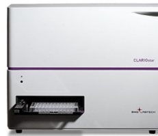
Clariostar , High Performance Scanning Multi-Mode Elisa & Microplate Reader. Possible Readings : Abs, UV-Vis, FI, FP, TRF, TR-FRET, Lum
