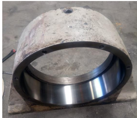
Recondition metal spray housing bearing
