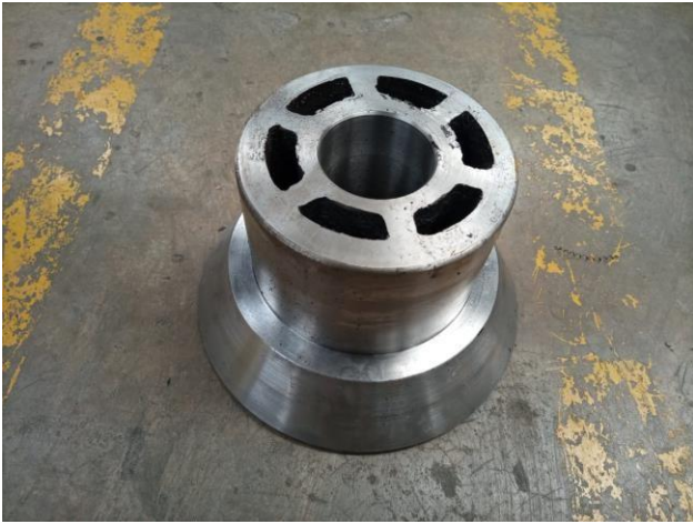
Fabrication roda crane
