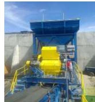
2016 - New Primary Crusher Cap. 500 TPH - PT. Muara Alam Sejahtera, Lahat, Sumsel
