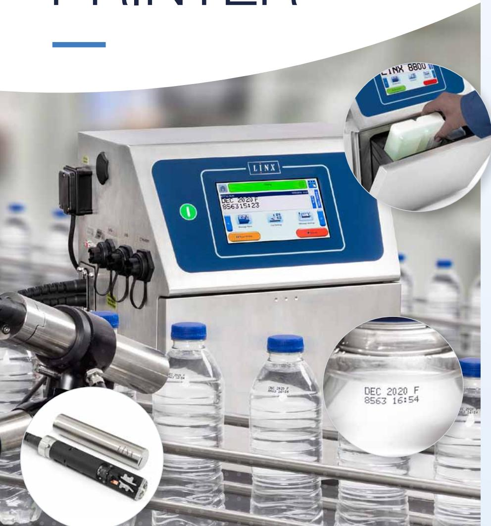
**The Linx 8830 continuous ink jet printer prints up to 3 lines and provides a perfect coding solution for industrial environments.**
