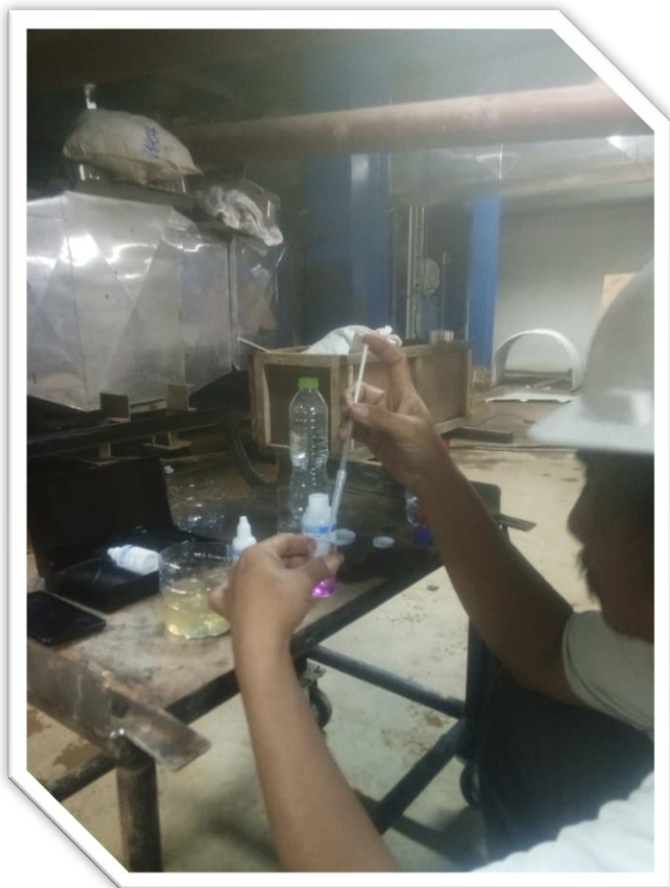
MEASUREMENT SAMPLE OF BOILER WATER
