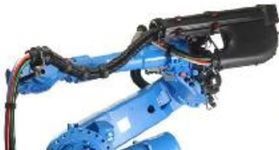
Solution 1: Energy conduit system with R-TecBox
