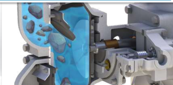
Large solids easily pass through pump
