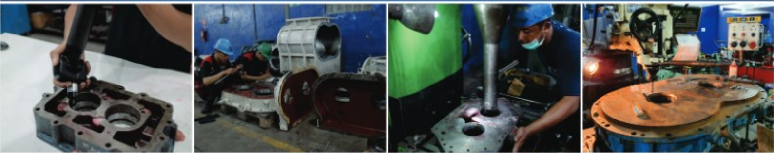
Sideplate, Bearing Housing Analysis & Repair Process
