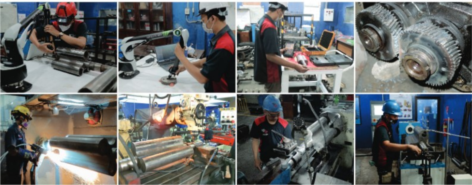
Roots Blower Rotor Gear, Analysis, Repair & Balancing Process
