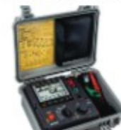
Insulation Test 12 KV
