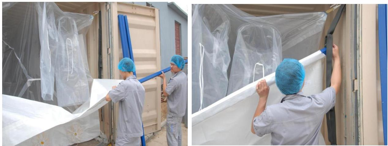
7 The remaining 3pcs steel bar fixated well, adjust the position well make the bottom steel bar cannot block the discharge spout.
