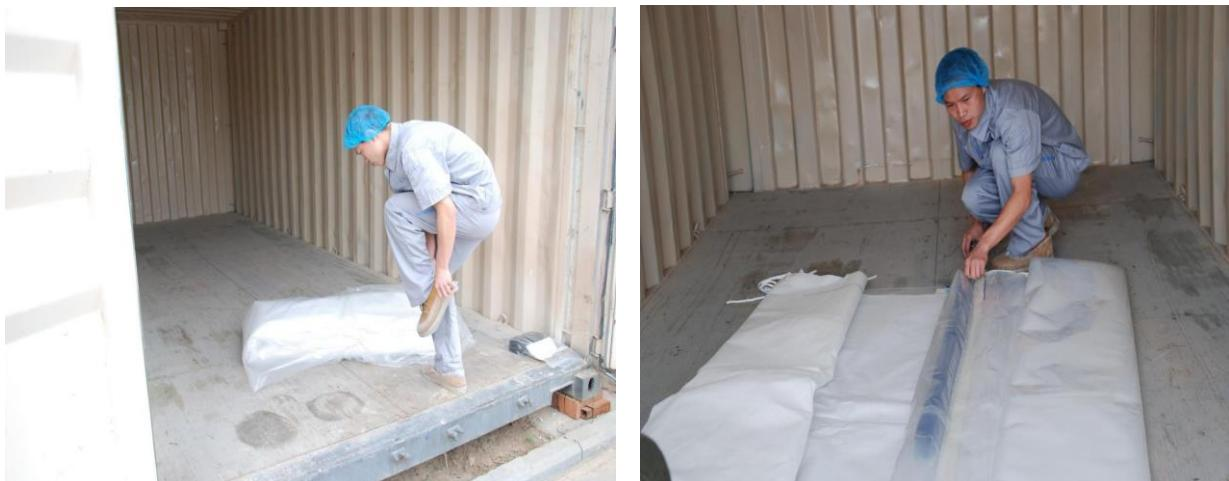
3 Set up the steel bar to the front sleeve horizontally into the container's trough
