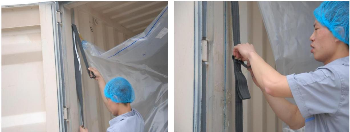
6 From the bulkhead sleeve fit with the first steel bar.
