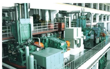
Gk270 密炼机 GK270Mixing machine
