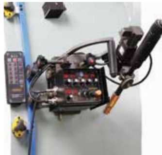
CS-51WE filet with Weaving welder for vertical-up
