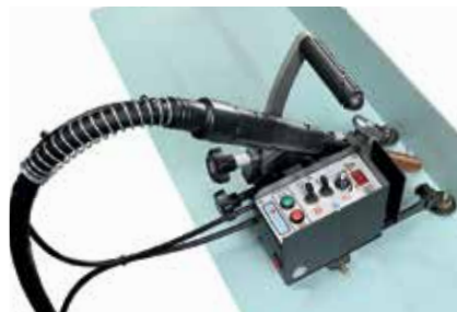
CS-71 fillet stitch continuous welder, Light weight
