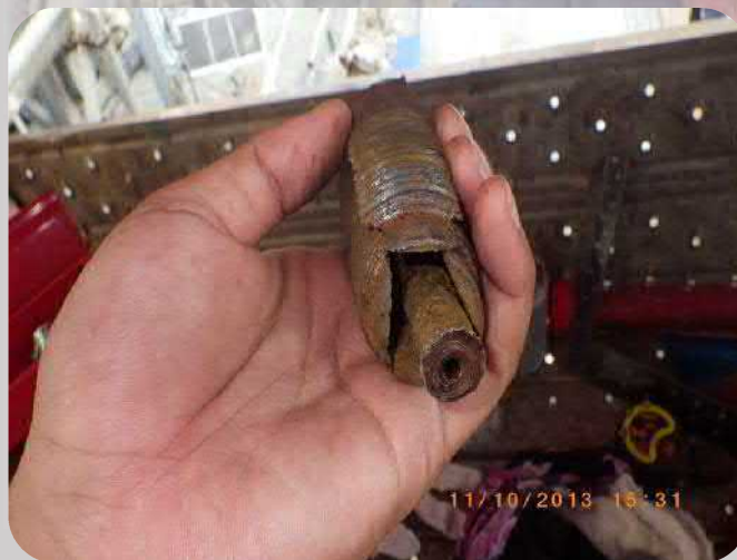
Spark Erosion, "Breach Closure 13-E-101A/B PCM TH" (PERTAMINA RU6, Balongan) 2013
