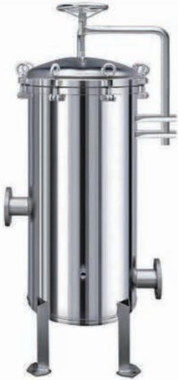
**DL Series** Stainless Steel High Flow Multi Cartridge Filter Housings are designed for processes requiring significant flow rate. The hand crank makes top cover removal and element change out quick and easy. These housings are suitable for a wide range of liquid processes and is able to accept different cartridge end cap styles in DOE and SOE.
