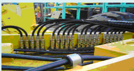
Vehicle auto lubrication system showing a pneumatic driven injector system installed on a motor grader construction equipment.
