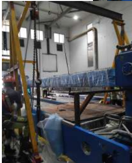
PT SMART TBK Pergantian cylinder press filter Andritz
